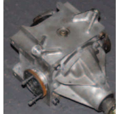
LEFT & BELOW The new Elite MX200 differential for the 2008 motorcycle-engined cars, above. Below, the original ADR-designed and built differential
