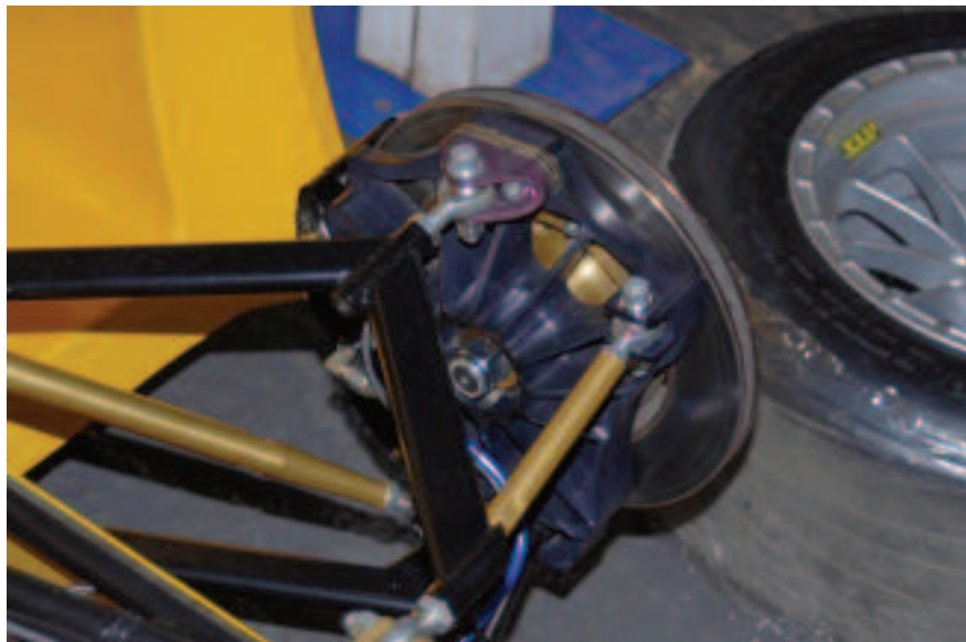
BELOW The front corner detailing the upright machined from aluminium alloy
